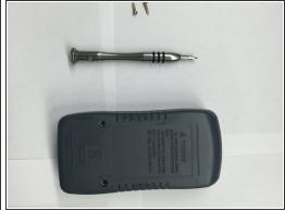
Turn over the DVM and unscrew the two screws using a J1 bit.
