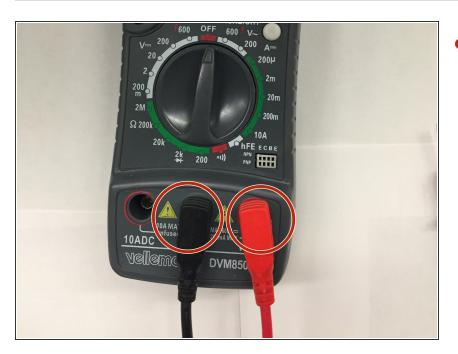
Remove lead connectors from front panel.
