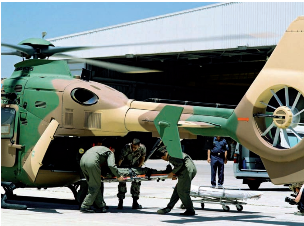
EC635 in Medical Evacuation mission: easy loading of the patient by the rear clamshell doors
