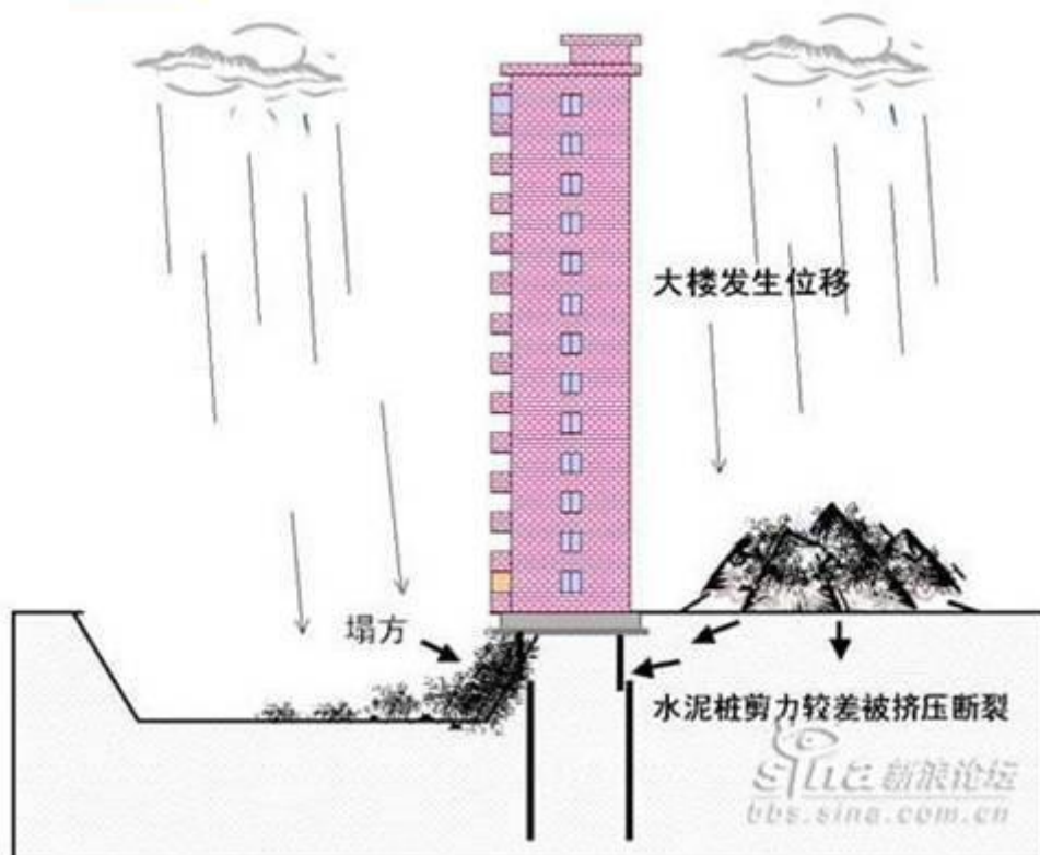
The building began to shift and the concrete pilings were snapped due to the uneven lateral pressures.
